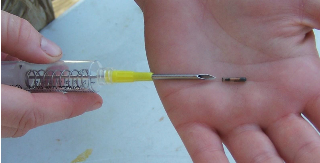
Photo 1. Typical PIT tag and injection needle. Small 0.47 inch (12 mm) long PIT tags will be used to monitor fish passage in Eagle Creek due to the relatively small size of fish to be tagged (4-10 inches long).
