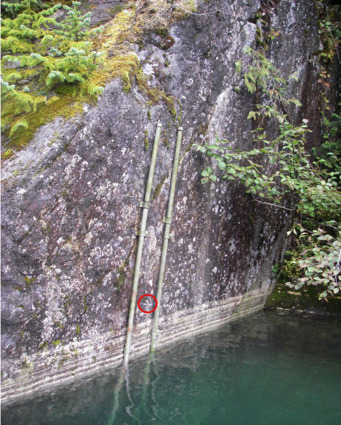
Picture 1. Turner Lake transducers and RM1 (circled in red). Lake level at 8.32 feet on September 30, 2010.
