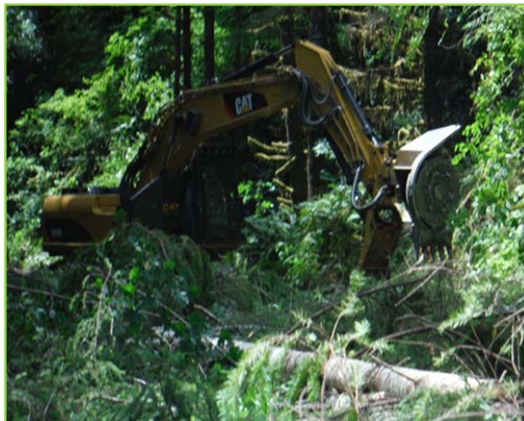
Excavator had a grinder head to mulch limbs
