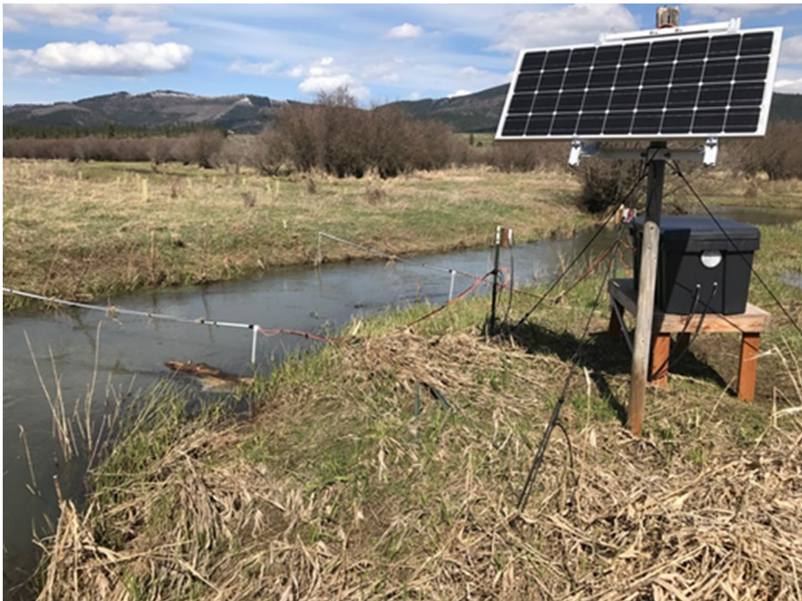
Picture 6. Portion of the newly activated relict channel and a PIT tag monitoring station after restoration was initiated, April 2017. This monitoring station was installed to determine migration timing and rearing locations of fluvial redband trout within the project reach. Protected tree plantings are in the background of the photo.
